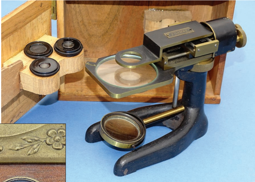
9. RARE FULLY-GEARED STAND FROM LYON, French, early 20th century, signed on a plaque “Instruments de Précision, J. Gambs, 8 Pl. des Jacobins, Lyon,” and on the oculars “J. Gambs, Lyon.” At minimum height this all brass microscope stands 4-3/4” (12 cm) tall, a narrow 2-1/2” (6 cm) wide and 6-5/8” (17 cm) long. The integral curved base and
