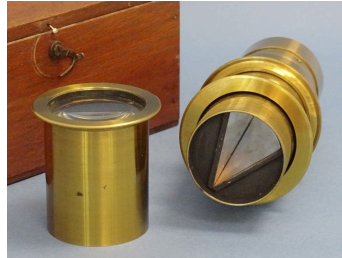
20. RARE KALEIDOSCOPIC PROJECTOR, English, c. late 19th c. This fine "magic" lantern projector is constructed of mahogany, bright lacquered brass, and japanned black sheet steel. The
