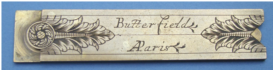
26. ELEGANT LEVEL / RULE BY BUTTERFIELD , French, c. first quarter 18th c., signed "Butterfield à Paris." This brass pocket instrument is 3-5/8" (9 cm) long (closed), with lovely decorative engraving on both sides. It opens, with a shaped strut, to form a right angle as well as a level with its plumb suspension hole, index line, and chamfered feet. It opens fully to form a half-the-King's-foot rule subdivided in inches ("pouces") and twelfths ("lignes"). In excellent condition, a fine merging of art and science. $895.
