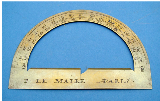
P. LE MAIRE A PARIS on a 3-3/4" (10 cm) wide brass protractor divided every degree from 0 to 180 and back, dating c. 1720. The maker was Pierre LeMaire senior (1695 - 1745), a splendid craftsman of quality instruments of science (see Rocca in SIS Bulletin , 2012).
