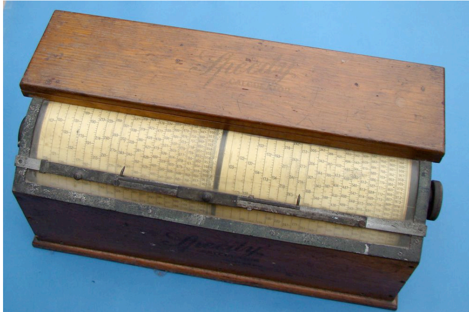
Catalogue 48. THE “SPEEDY CALCULATOR” -- A SEEMINGLY UNRECORDED SPIRAL SLIDE RULE , c. early 20th century, signed three places on the wood housing “Speedy Calculator, Bté. S.G.D.G.” Measuring 19” (48 cm) wide overall, the calculator has a golden oak housing, celluloid window with cursor line, twin pointers on double metal slides, external button, and two large logarithmic drums, independently rotatable. Condition is good, the drum rotation now quite tight. The machine apparently uses twin drum scales in direct analogy to twin sliders on a straight in-line slide rule, for all matters of multiplication and division. Possibly of French manufacture for the English market (or vice-versa ?), we find no example of this machine in the catalogues of the Science Museum and C.N.A.M. collections, nor any record in the standard literature, including Cajori’s comprehensive list. $2850.
