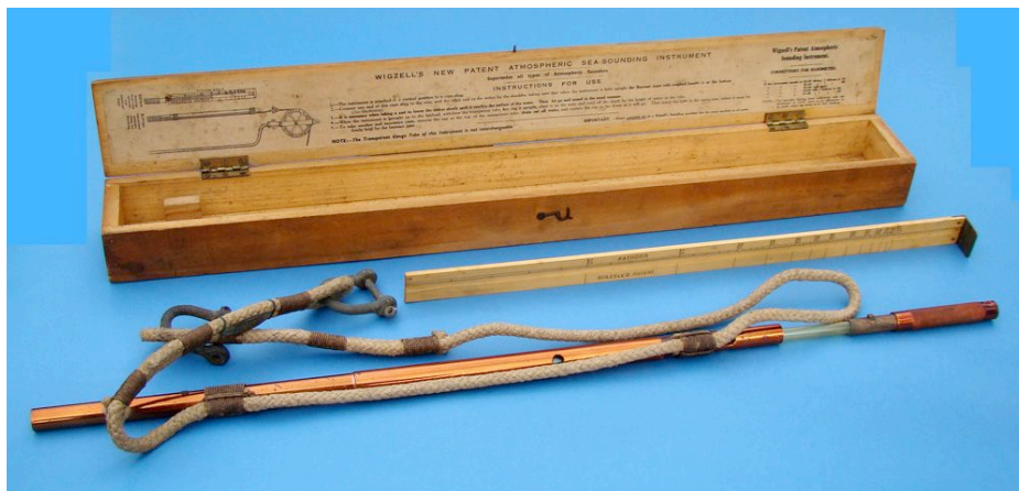
Catalogue 53. WIGZELL'S SEA SOUNDER , English, early 20th century. Contained in the original 27" (69 cm) long wood case is the metal sounding tube with internal transparent tube, rope sling with shackles for attachment to a sounding wire and to a sinker weight, wood rule calibrated with fathom scale (from 5 to 100 fathoms), and instruction label with barometric corrections. The system permits accurate depth sounding based on the compression of air in the tube by the pressure of water at depth. In fine condition. $1250.
