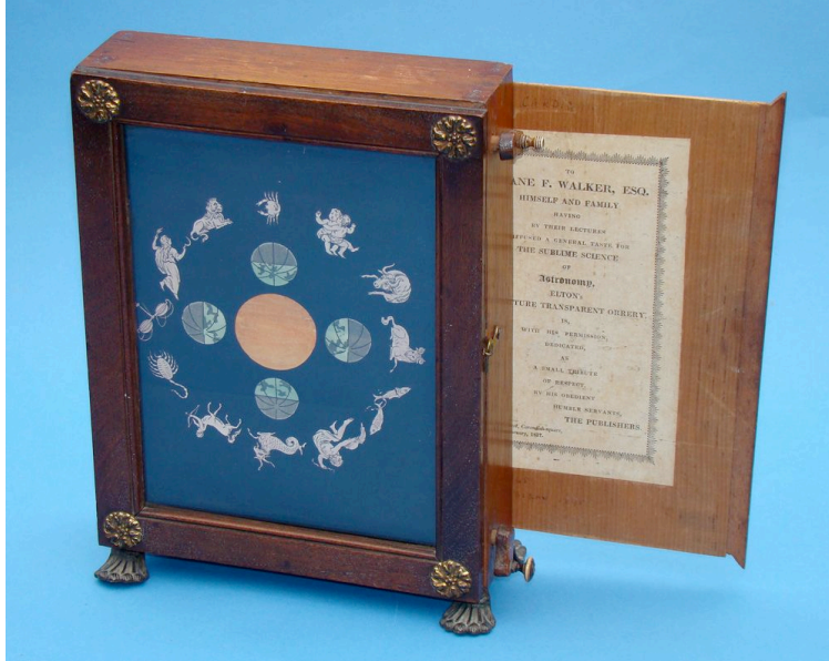
Catalogue 18. ELTON'S TRANSPARENT ORRERY -- AN ASTRONOMICAL SCROLL , English, c. 1820. The paper scroll is hand-colored with seven images of the solar system, eclipses, Orion, etc. It is driven by two ivory handled cranks, and housed in a mahogany stand 8" x 10" x 3" (20 x 25 x 8 cm) overall, with gilt brass mounts and feline feet. The front is glazed and hinged, the back removable for using a candle, etc., as rear illumination of the transparent illustrations. A trade label on the back dedicates Elton's orrery to "Deane F. Walker, Esq., himself and family, having by their lectures diffused a general taste for the Sublime Science of ASTRONOMY." This rare device is in very fine condition, except for some minor repairs to, and possible incompleteness of, the long scroll. $5800.
