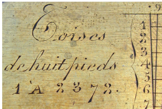
Catalogue 30. UNUSUAL SURVEYOR'S OR ARCHITECT'S RULE , probably French, early 19th century, signed in lovely script "Clavel Jn-Pierre, Géomètre Mésureur." The 7-1/2" (19 cm) long brass rule has scales on both sides for equal parts, with interpolation grids, in both old and new measure. Included are "Toises de 8 pieds (1:2500), Mètres (1:2500), Decimètre Naturel, Toises de huit pieds (1:2372), Mètres (1:2372)" and the unusual "demi pied de Chambre." Condition is fine, noting general wear to the surface. The curiously named "pied de Chambre" was equal to the pied de Savoie, and was used in particular by carpenters in the entire Duchy of Savoy. The maker Jean-Pierre Clavel, although unrecorded in the standard references, produced this splendid rule with an exquisite style of engraving. $1450.
