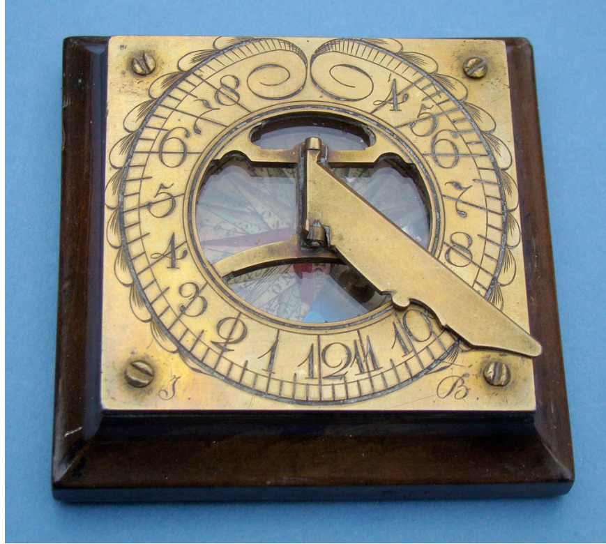
Catalogue 27. MINIATURE TABLE DIAL BY BERINGER , German, late 18th century, signed "JB." The 2-1/2" (6 cm) square brass dial plate is mounted on a shaped wood base with brass feet, and contains a glazed compass with hand-colored paper rose. A shaped folding gnomon casts its shadow on the beautifully engraved chapter ring. The maker was apparently the elusive J. Beringer, close relative of David Beringer of Nuremberg. A lovely dial in fine condition, all original, a very rare example of this maker's work. $1350.
