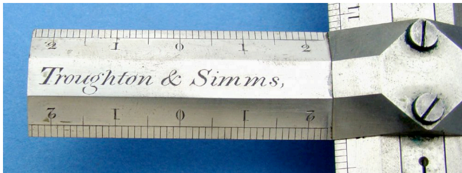
Catalogue 13. TWIN PRECISION ORTHOGONAL PLOTTING RULES IN ELECTRUM , English, 2nd quarter 19th century. These splendid rules measure 12" (30 cm) long, with a 5" (13 cm) sliding crossbar. Rule and crossbar are divided along each edge, permitting rapid graphical plotting or readout. One has scales of 2 (also 6) "inches to a mile in feet," the other 2 (also 2-1/2) "chains to an inch." Beautifully constructed in silvery electrum alloy, these unusual rules are in pristine condition, in their original velvet lined mahogany case. $1750.
