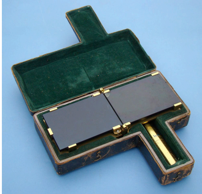
Catalogue 50. FRESNEL MIRRORS FOR INTERFERENCE OF LIGHT , probably Continental, c. second quarter 19th century. The two front surface mirrors are made of thick black glass held in a precision mount of bright lacquered brass, 7-3/4" (20 cm) wide. The mirrors are spring-loaded against three thumbscrews for fine adjustment of tilt. There is a hinged mounting bracket to the rear.
