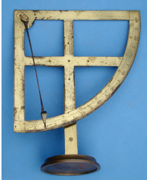
Catalogue 12. FINE STANDING ASTRONOMICAL QUADRANT , probably English, mid-18th century. This finely made brass quadrant, with radius of 8-1/4" (21 cm), is equipped with a weighted pointer on a swinging steel arm. The offset buttressed brass support arm is now mounted on a circular brass base. The quadrant scale is divided every 1/2°, and finely engraved every 10° from 0° to 90° and back again, with decorative divisions every 5°. It is likely that the present quadrant could be used on, for example, a large telescope or other sighting instrument, to indicate star elevations, etc. Much larger versions are discussed by Bion, equipped with their own permanent mounting brackets and telescope swinging in a vertical arc. An uncommon instrument, in fine condition. $3200.
