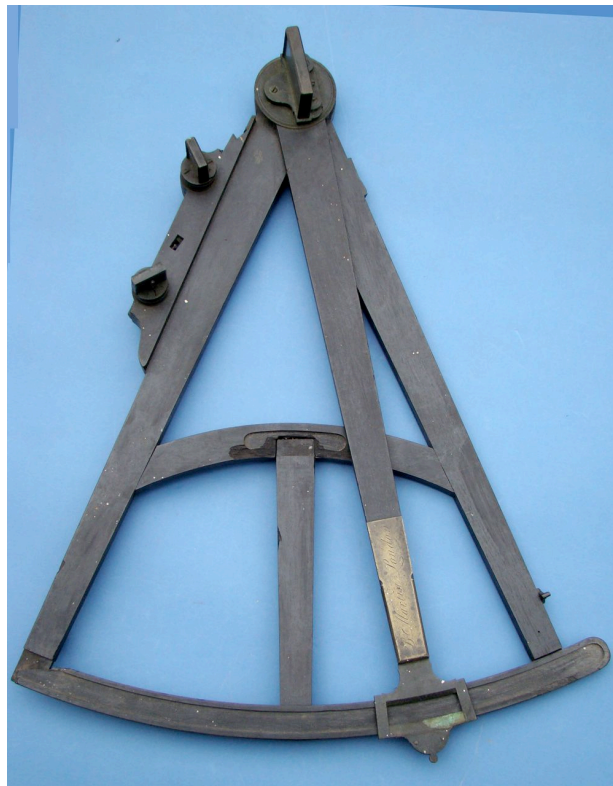
B. Martin, London on the brass terminus of the ebony index arm on a large (20" or 51 cm overall) but quite incomplete ebony octant. It dates c. third quarter 18th century, and is a rather rare example. Martin later joined with his son and was granted a patent for an improved octant featuring an index arm mirror easily adjustable about two axes (see Tesseract Cat 44 Item 23).
