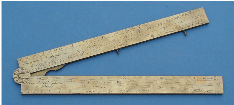
Catalogue 11. FINE CHEVALLIER SECTOR, French, c. 1800, signed “Chevallier, Ingr. Opticien, de S.M. le Roi de Westphalie à Paris.” The brass sector opens to 13” (33 cm), and is finely engraved with scales for polygons, chords, solids, metals, equal parts, weights of shot, calibers of cannon, etc. The maker is probably Jean-Gabriel-Augustin Chevallier, working at the corner of Pont-Neuf and the quai de l’Horloge, at the sign “L’ingénieur Chevallier.” Fine condition, and beautifully engraved, by maker to His Majesty the King of Westphalia. $1350.
