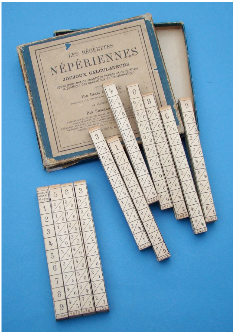
Catalogue 72. “LES RÉGLETTES NÉPÉRIENNES,” French, c. 1885, the set of ten true Napier’s rods made of wood sticks 4” (10 cm) long covered on all four sides with printed paper scales, by Genaille and Lucas, in very fine condition housed in the original somewhat worn box with original printed label and instructions. These Napier’s “bones” permit easy multiplication of multi-digit numbers. Very rare, even rarer than the rod designs invented by Genaille. $2800.
