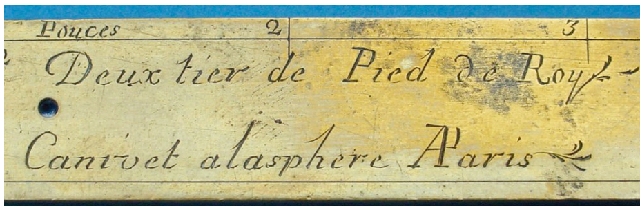
Catalogue 83. GEOMETRICAL CHORDS ON A FOLDING RULE, French, second half 18th century, signed “Canivet à la sphère à Paris.” This finely crafted folding brass square opens to 4-1/2” x 4-1/2” (11.4 cm), and has a charming scale of French inches (“Pouces”) and twelfths (“lignes”) labeled “Deux tier de Pied de Roy” (i.e., “Two-thirds of the King’s foot”, although this is a mistake, as in reality the length is one-third of the King’s foot). The other arm is engraved with a 60° arc of a circle subdivided every 5°, the ranges 0° - 10° and 50° - 60° further subdivided every 0.5°. Using a pair of dividers gives the lengths of chords of a circle (of radius 3.18 French inches, determined here by simply measuring the 60° chord length). Linear scales of chords are frequently applied to sectors, Gunter’s rules, surveying alidades, etc., but we note only one other instance of the arc laid out directly on a rule, that on a reigle platte (Tesseract Catalogue 78 Item 31). Scales and labels are very finely engraved. Condition is fine noting a little pitting. $1400.
