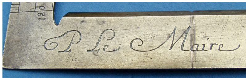
P. Le Maire A Paris on a 3-3/8" (9 cm) wide brass protractor divided every degree from 0 to 180 and back, dating c. 1720. These two Pierre le Maire (senior) signatures show an
