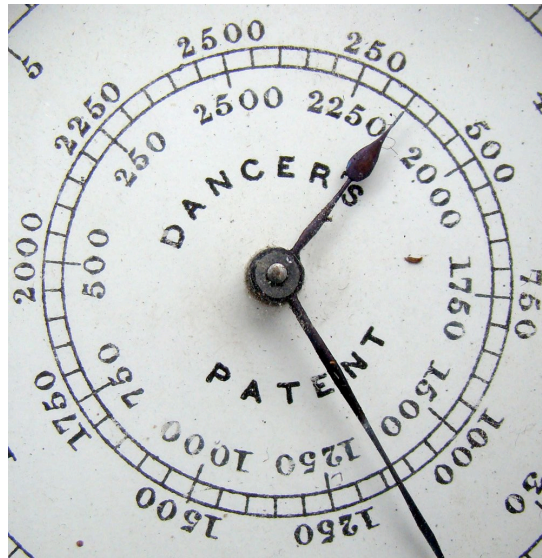
Catalogue 31. DANCER'S PATENT SPEED INDICATOR , English, c.1870. With gearwork contained in a fine lacquered brass housing 2-1/2" (6 cm) in diameter, this form of odometer permits accurate measurement of the speed of machinery. It is complete with friction wheel, toothed wheel, adjustable stabilizing guide, and push-button release mechanism. The patent (1867) holder, and probable maker, was John Benjamin Dancer, "Mathematical Instrument Maker" of Manchester, famous for his microphotographic slides and ingenious mechanical devices. A very rare instrument, in very fine condition, complete with original mahogany case. $1950.
