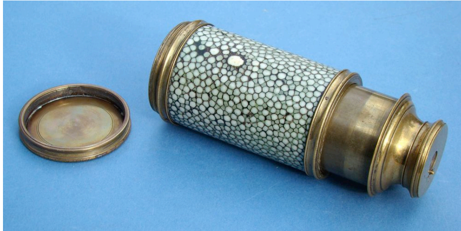
Catalogue 71. FINE RAYSKIN-COVERED TWIN-POWER MONOCULAR , English, late 18th century. Opening from 3-1/2" to 5-1/4" (9 - 13 cm), the brass telescope has Galilean optics with a fine triplet objective, twin eye lenses on a swivel mount separated by dust stop, and replaced dust cover for the objective. The main tube has its original beautiful green rayskin binding. A lovely telescope in fine condition. $1150.
