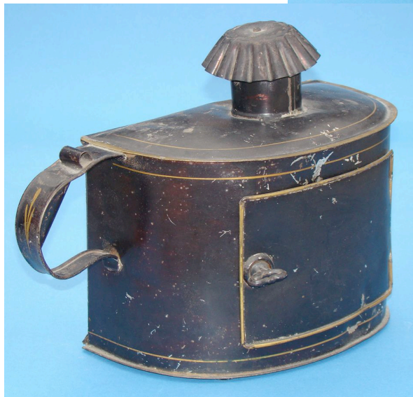
Catalogue 15. CLARKE'S ASTRONOMICAL CANDLE-LANTERN , American, c. 1875. This painted tin lantern measures 12" x 9"x 6" (30 x 23 x 15 cm) overall, complete with carrying handle, shaded smoke stack, hinged rear door, four candle-holders, and ground glass screen. A slot in front of the glass would accommodate various perforated cards of star patterns, for comparison with the night sky. Patented in 1870 by James Freeman Clarke of West Roxbury, Mass., the Astronomical Lantern is an unusual example of Yankee ingenuity. Clarke (1810 - 1888) was a noted author, clergyman, and Harvard professor. This lantern is in good condition, noting a few dents and scrapes, and a crack to the glass corner. It retains its original paint decoration. $950.
