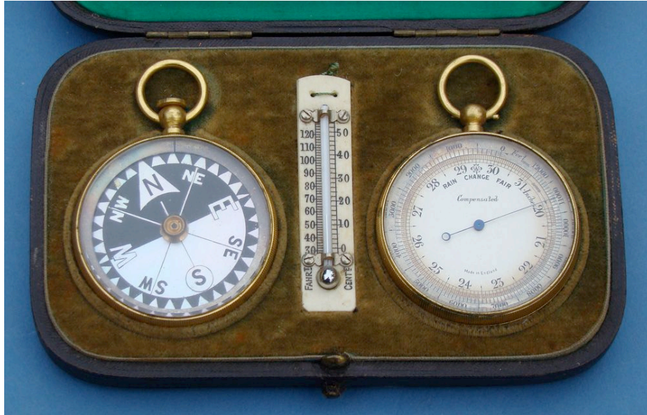
Catalogue 79. FINE EXPLORER'S COMPENDIUM , English, c. 1900, the 5-3/4" (15 cm) wide case containing a glazed watch case compass with floating mother-of-pearl compass "card" and gilt body; an ivory mounted thermometer with Fahrenheit and Centigrade scales; and a matching gilt watch case barometer with rotatable altitude scale. The case is bound in red Morocco leather and lined in green silk and velvet. Condition is very fine throughout. $950.
