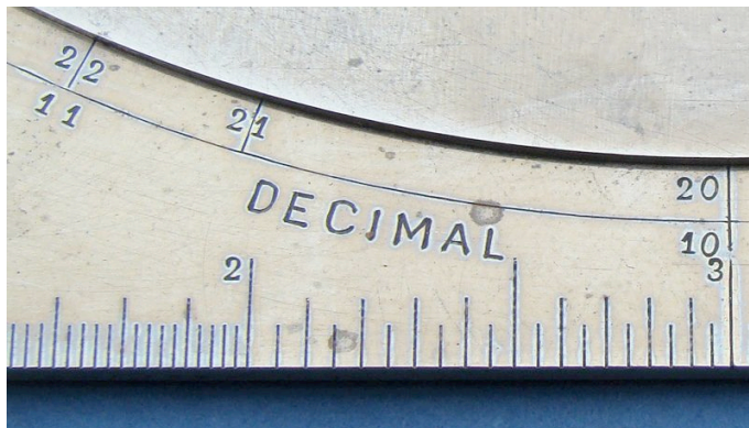
Catalogue 17. MULTIPURPOSE MATHEMATICAL TOOL , English, second half 19th century. Made of electrum 6-1/2" (16.5 cm) square, this plotting tool has a fine central rotating protractor with one arcminute vernier, edge scales of sines, cosines and logarithms, and circular scales for direct angular conversions labeled for single digit fractional multipliers, decimal multipliers, and for different displacement-to-length ratios. Finely made and in fine condition, the only example of this device we have seen. $1450.
