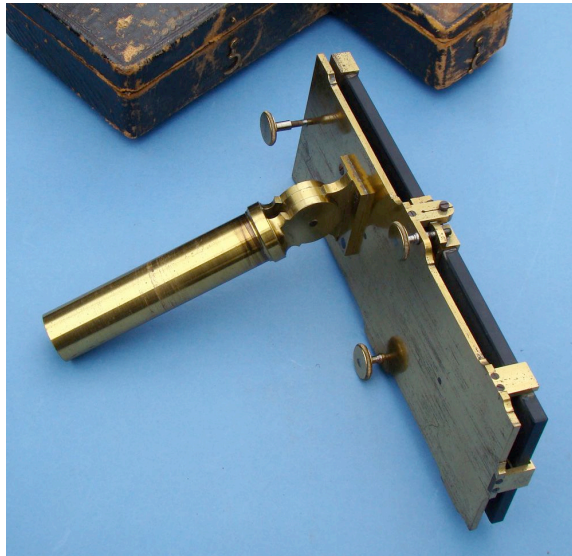
Catalogue 50. FRESNEL MIRRORS FOR INTERFERENCE OF LIGHT , probably Continental, c. second quarter 19th century. The two front surface mirrors are made of thick black glass held in a precision mount of bright lacquered brass, 7-3/4" (20 cm) wide. The mirrors are spring-loaded against three thumbscrews for fine adjustment of tilt. There is a hinged mounting bracket to the rear.
