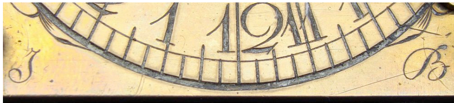
Catalogue 27. MINIATURE TABLE DIAL BY BERINGER , German, late 18th century, signed "JB." The 2-1/2" (6 cm) square brass dial plate is mounted on a shaped wood base with brass feet, and contains a glazed compass with hand-colored paper rose. A shaped folding gnomon casts its shadow on the beautifully engraved chapter ring. The maker was apparently the elusive J. Beringer, close relative of David Beringer of Nuremberg. A lovely dial in fine condition, all original, a very rare example of this maker's work. $1350.
